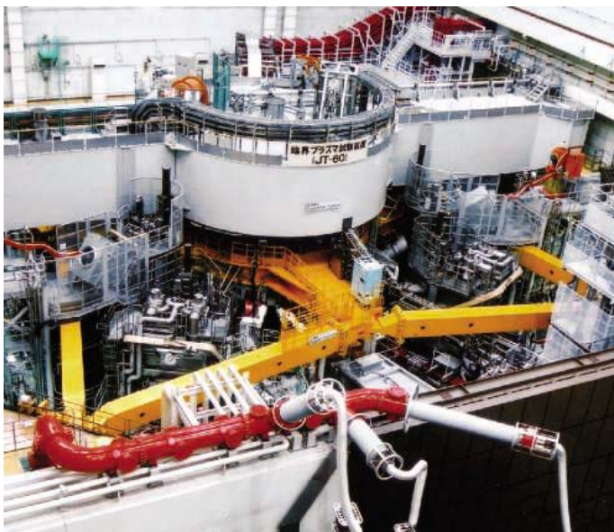
Reactor reborn. Japan will remove the core of its JT-60 reactor and rebuild it with superconducting magnets to aid the ITER project.
